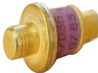
Figure 2(a) : Gunn diode Characteristics (b): Gunn Diode
