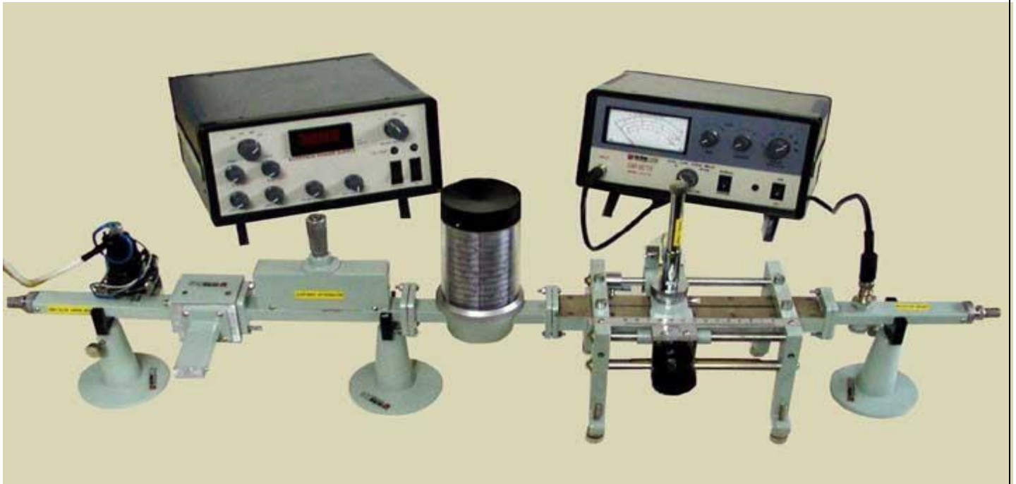
Figure.2 Microwave bench set up
